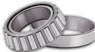
All Heavy Duty Wheel Bearings have tapered rolling-element bearings which are designed to provide higher load carrying capacity in both directions to handle vertical and axial loads. They also feature crowned raceways and precision matched rolling elements for even load distribution. They are manufactured with premium quality steel for greater machining and high strength.
