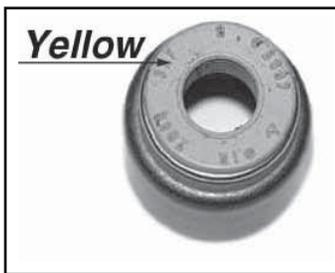
**Intake Valve Stem Seal**
