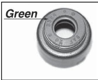
**Exhaust Valve Stem Seal**
