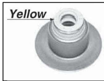
**Intake Valve Stem Seal**
