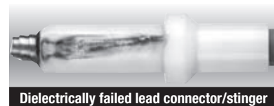
Dielectrically failed lead connector/stinger
